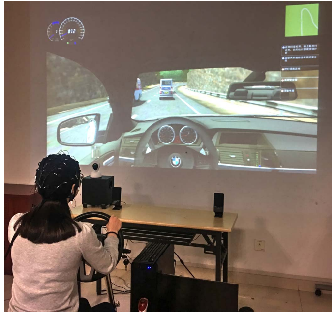
Fig. 1. Simulating experimental setup for obtaining EEG signals under alert and fatigue driving states.
