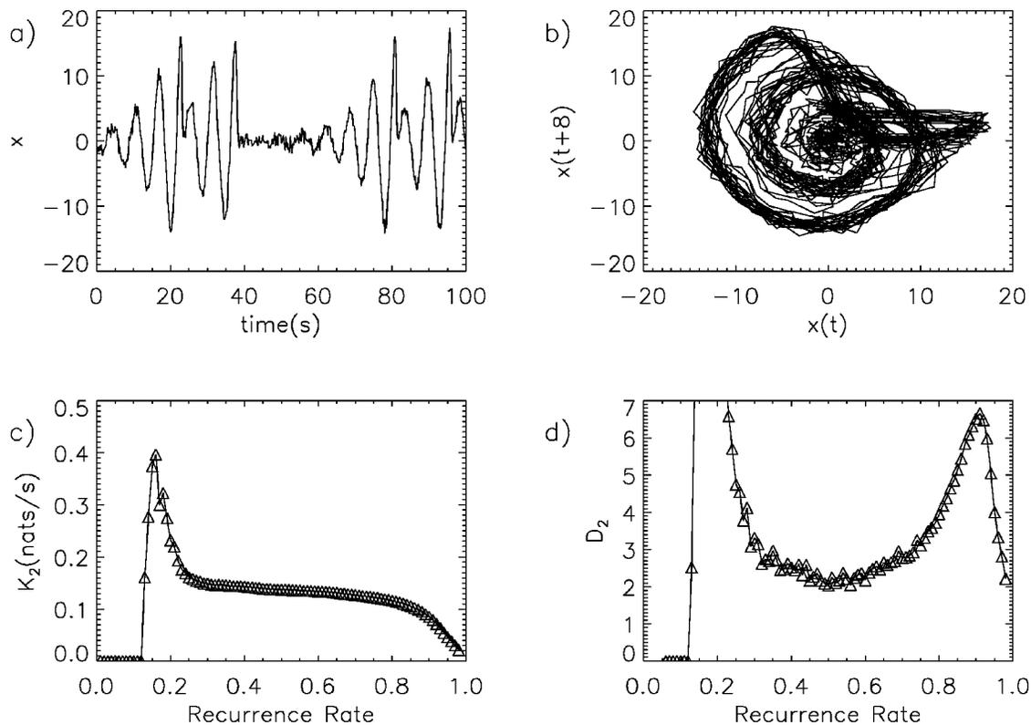
FIG. 8. (a) Sample of the time series of the Rössler attractor in the funnel regime ( $a=0.25$ ,  $b=0.4$ , and  $c=8.5$ ) with observational noise (10% of the standard deviation of the signal); (b) reconstructed attractor; (c) dependence of correlation entropy on the recurrence rate; (d) dependence of correlation dimension on the recurrence rate.
