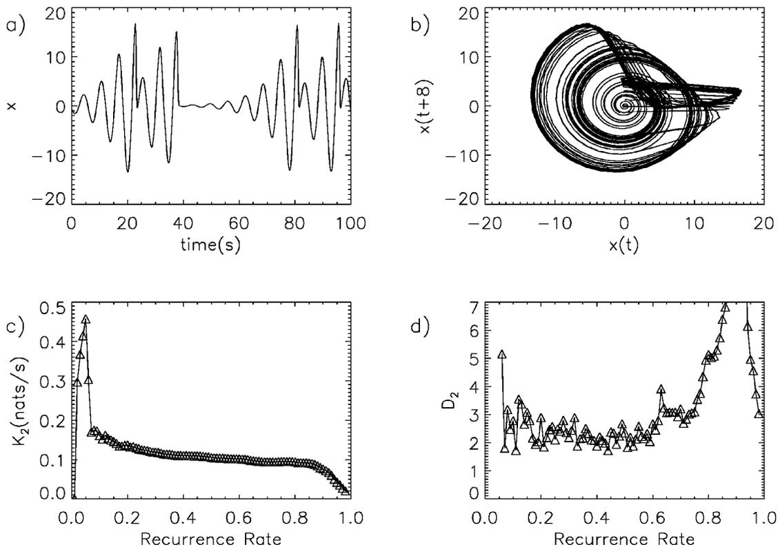
FIG. 4. (a) Sample of the time series of the Rössler attractor in the funnel regime ( $a=0.25, b=0.4, c=8.5$ ); (b) reconstructed attractor; (c) dependence of correlation entropy on the recurrence rate; (d) dependence of correlation dimension on the recurrence rate.
