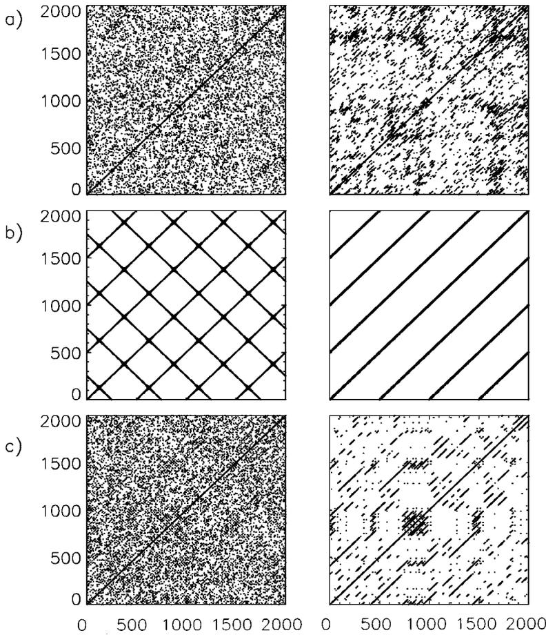
FIG. 1. RPs for uniformly distributed noise (a), the sine function (b), and the Rössler system (c). The left panel shows the plots for  $d=1$ . The right panel represents the plots for  $d=14$ ,  $d=2$ , and  $d=3$ , respectively, from top to bottom.  $\epsilon$  is chosen so that the recurrence rate (percentage of black point in the plot) is the same for the embedded and nonembedded time series.
