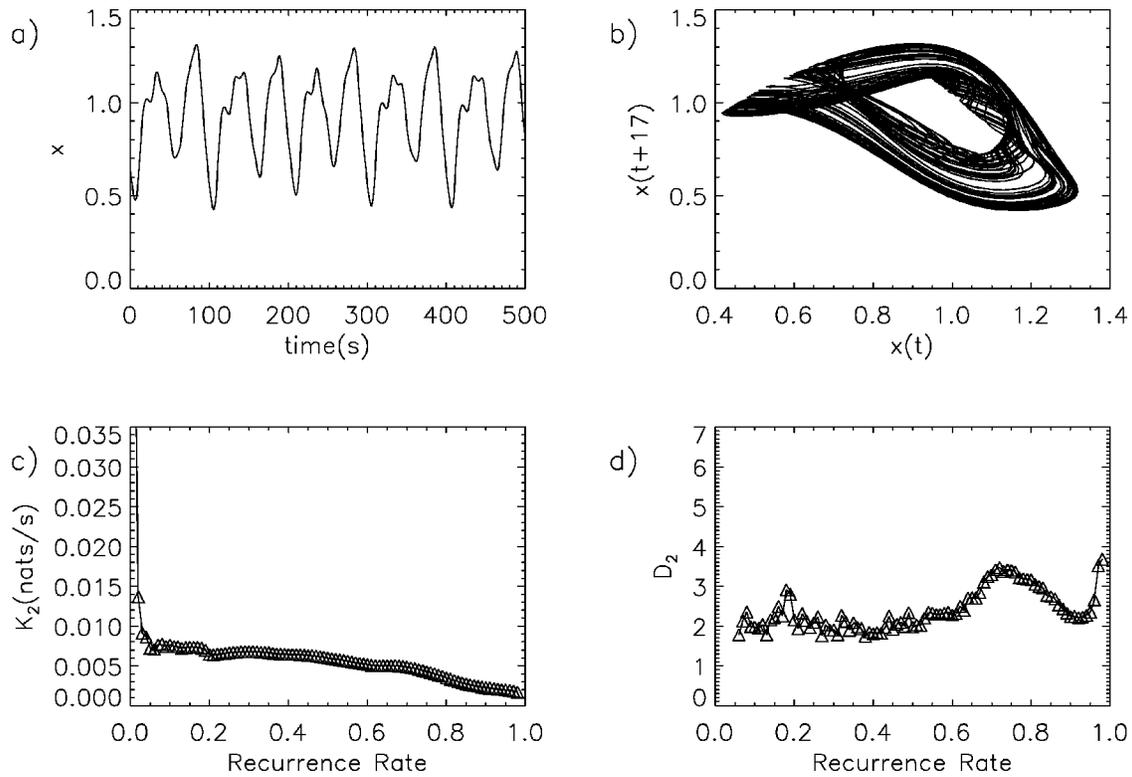
FIG. 5. (a) Sample of the time series of the Mackey–Glass system for  $\tau=17$  (chaotic regime); (b) reconstructed attractor; (c) correlation entropy in dependence on the recurrence rate; (d) correlation dimension in dependence on the recurrence rate.
